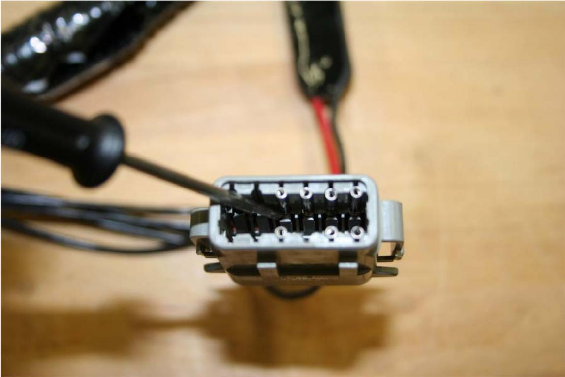
5) Insert the wires of the new power board into the gray connector as shown in the pictures below (yours may look like the left or the right picture). The blue wire goes to pin 2, the yellow wire goes to pin 9, and the black wire goes to pin 10. Push each in until it "clicks" and seats fully.
