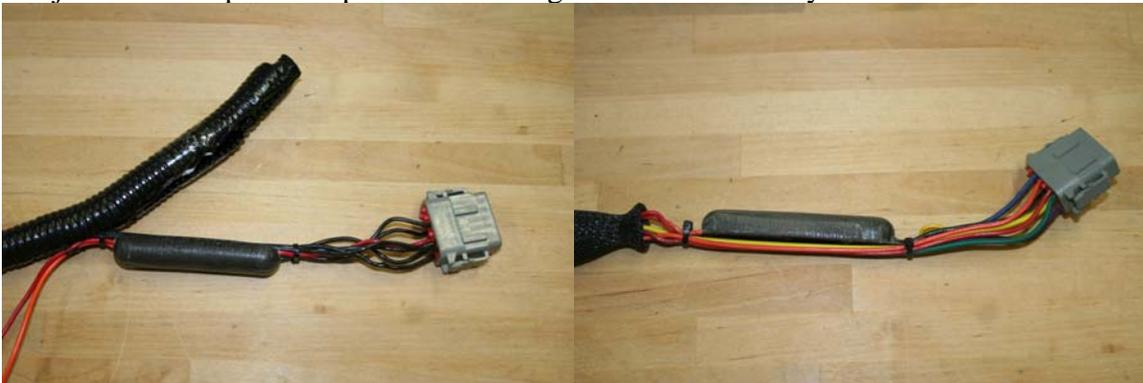
Next, cut the zip ties that hold the power board to the other wires.
