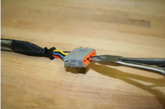
2) There are 2 types of harnesses, one uses loom (left picture) and the other uses expandable sleeving (right picture). If you have the loom type, you will need to cut the black wrapping tape to remove the old power board. If you have the sleeving type, you can just cut the zip tie and push the sleeving back out of the way.
